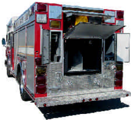
Ground Ladder Storage and Additional Hose
